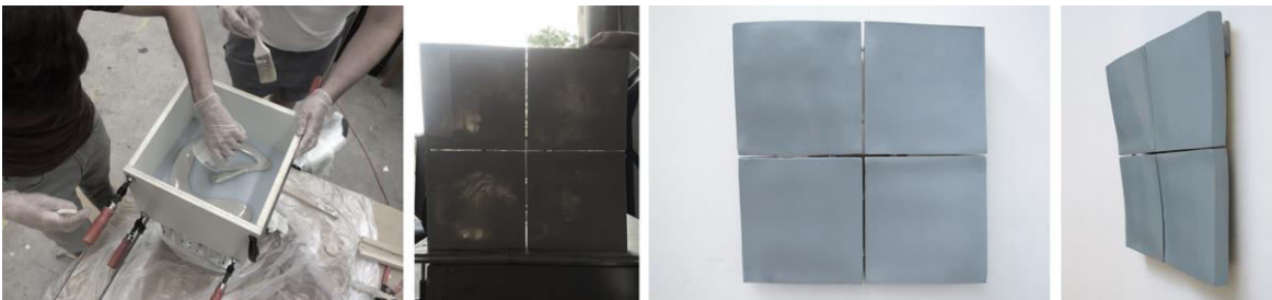
Figure 15: Test Two preliminary fiberglass resin panel test.
