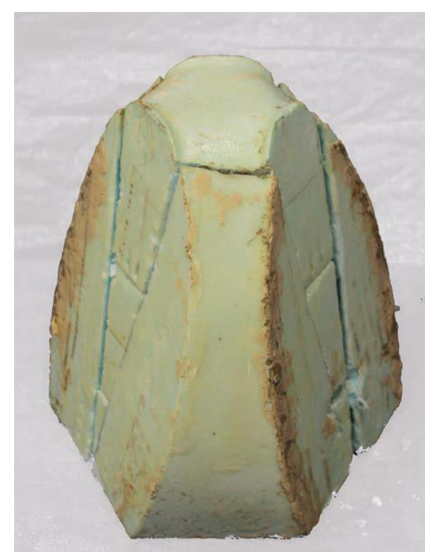
CENTER PIECE AFTER SLICING FOR REMOVAL FROM FORM.
