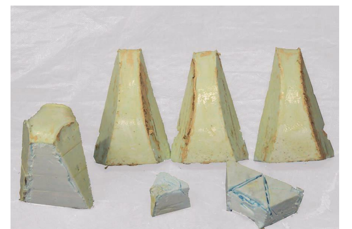
CENTER PIECE AFTER SLICING FOR REMOVAL FROM FORM.
