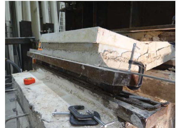
Shear in Panel
