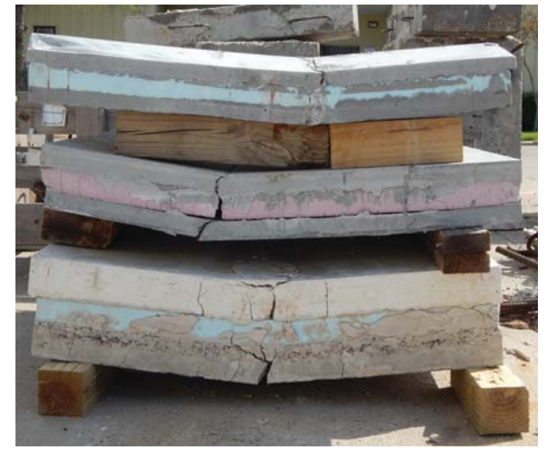
Panel 1, 2, & 3 After Structural Testing
