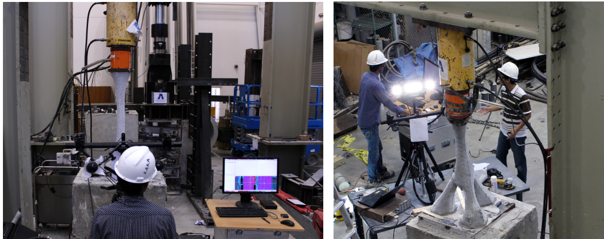
Figure 6. Load testing at UTA CELB: Column #1 (left) and Column #3 (right)
