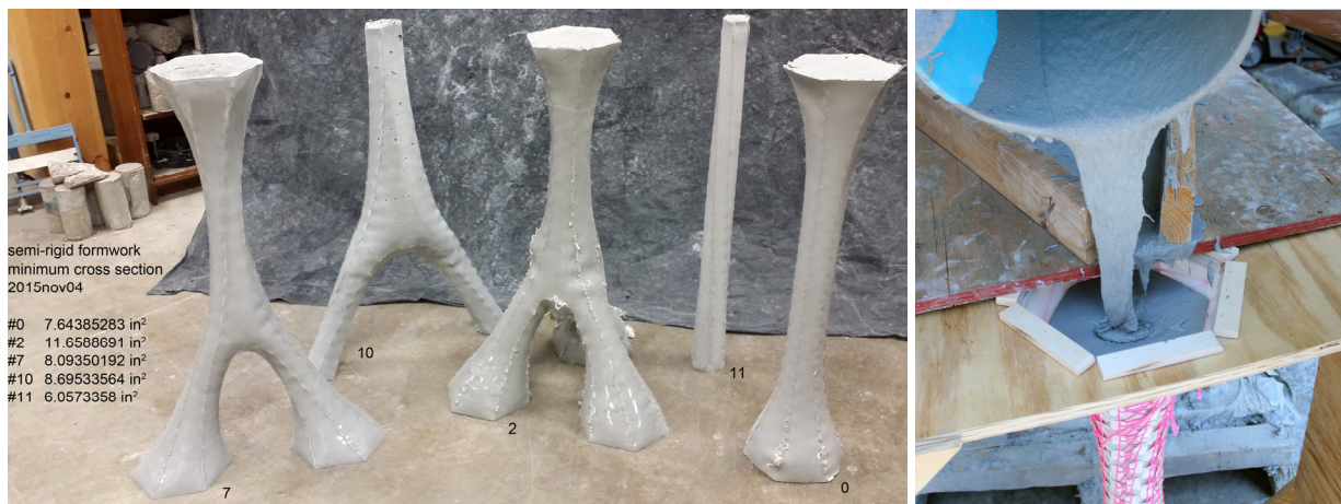
Figure 4. Five different columns with various non-Euclidean geometries and UHP-FRC
