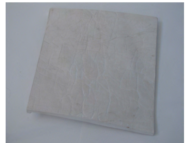
HYDROSTONE Panel with 1/8" Silicon and Unrolled Surface Paper to interpolate geometry at edge of mold.
