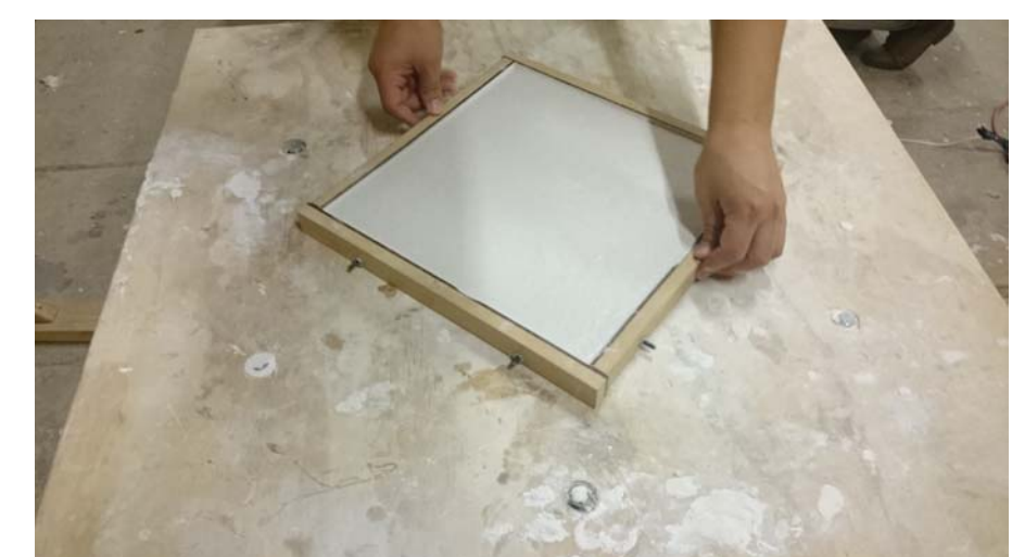
Mixture was vibrated on the vibrating table to level the mixture and release air bubbles.
