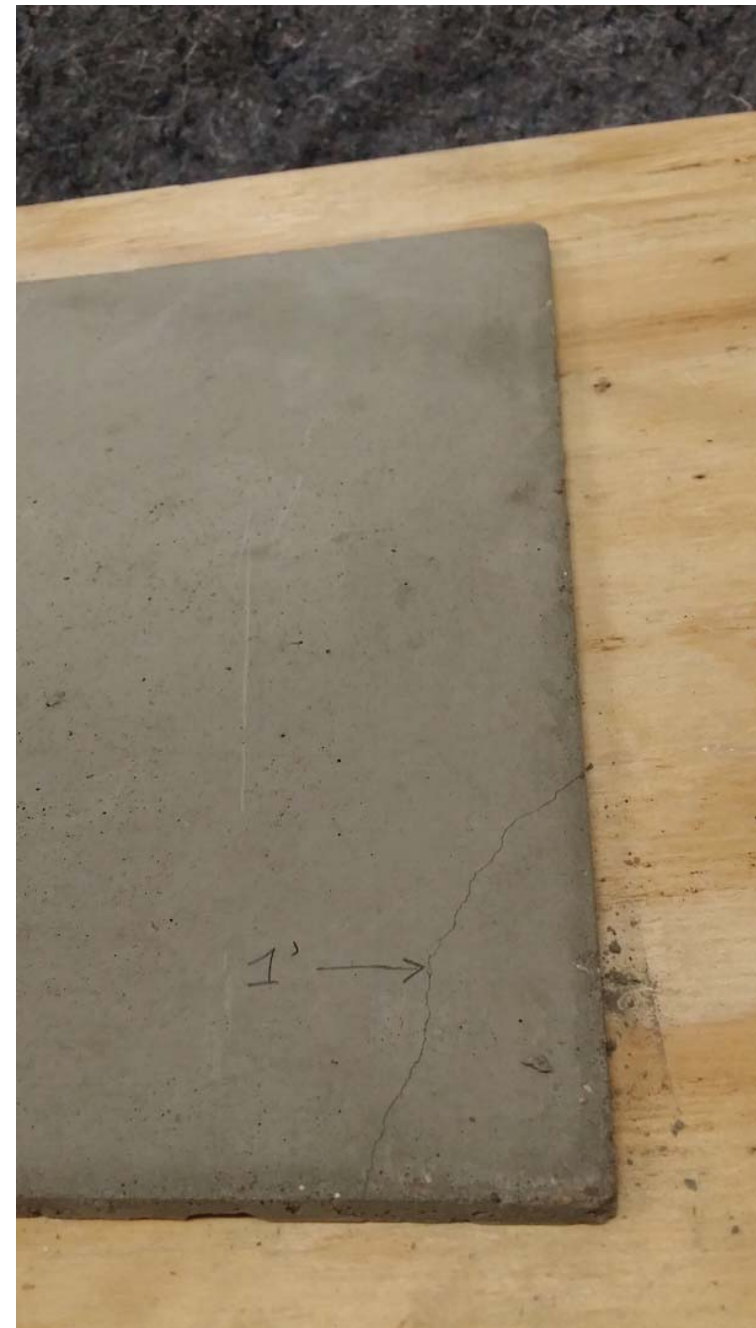
Concrete + Non-shrink Grout: 1 ft
