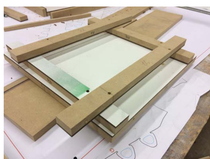
MDF was backed up with melamine to prevent MDF from absorbing moisture and for easy removal of the casted panels.
