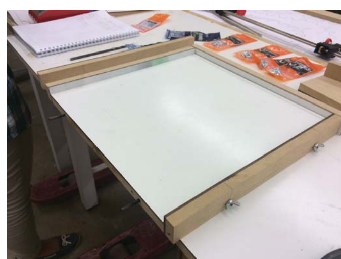
The pieces were bolted together to form the mold. Mold dimension: 12in (W) x 12in (L) x 0.5in (H)
