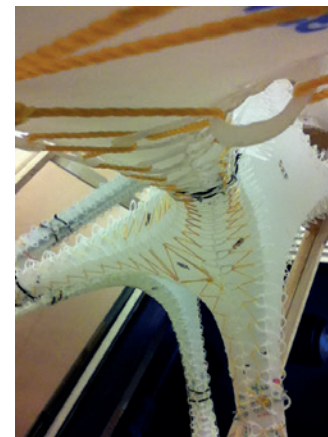
Fig. 11: Nylon string laced through tabs in plastic formwork. (Photo: Ken Tracy)
