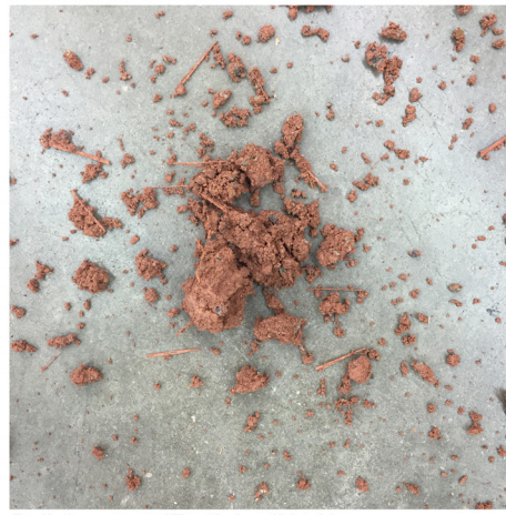
Ball drop test (Earthdwell Ltd.)
