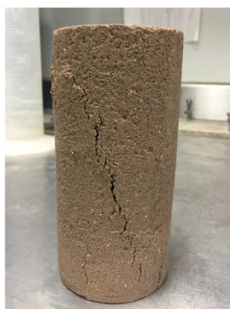
Sample A- ω=10.14% Maximum stress=16.3 psi
